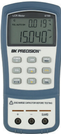
FIG. 11.27 Digital reading inductance meter. (Courtesy of B+K Precision)
