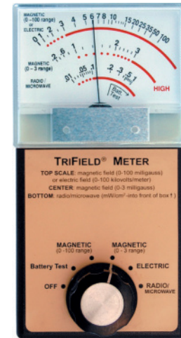
FIG. 11.14 Milligaussmeter. (Courtesy of AlphaLab, Inc.)
